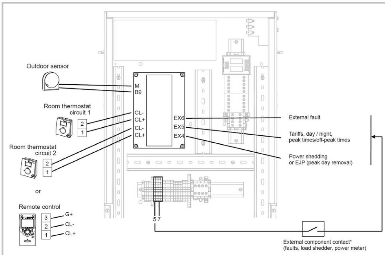
\* If the control device does not provide a potential-free contact, the contact must be relayed to create equivalent wiring. In all cases, please refer to the instruction manuals for the external components (load limiting device, power meters) to create the wiring.
