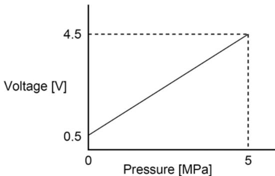
If the voltage is not correct, replace Pressure Sensor.
