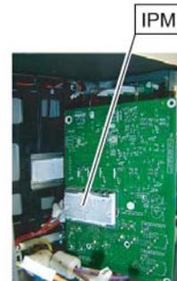
Spread the heat dissipation compound on the other side of IPM when you exchange PFC PCB by the repair.
