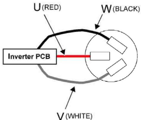
Check connection of inverter PCB
