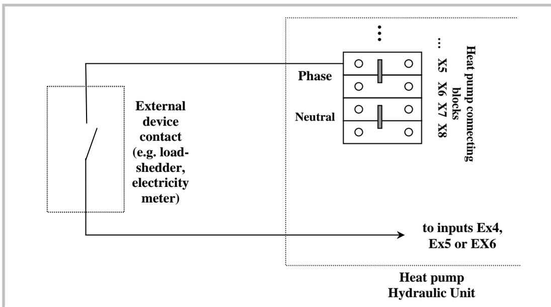
Figure 1: Typical Wiring of External Devices
