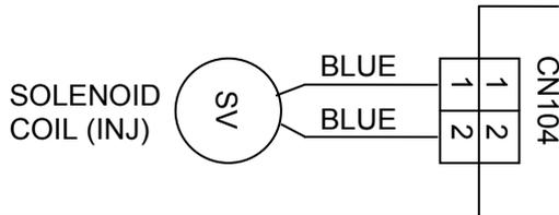
**Check point 2 : Check solenoid coil**
