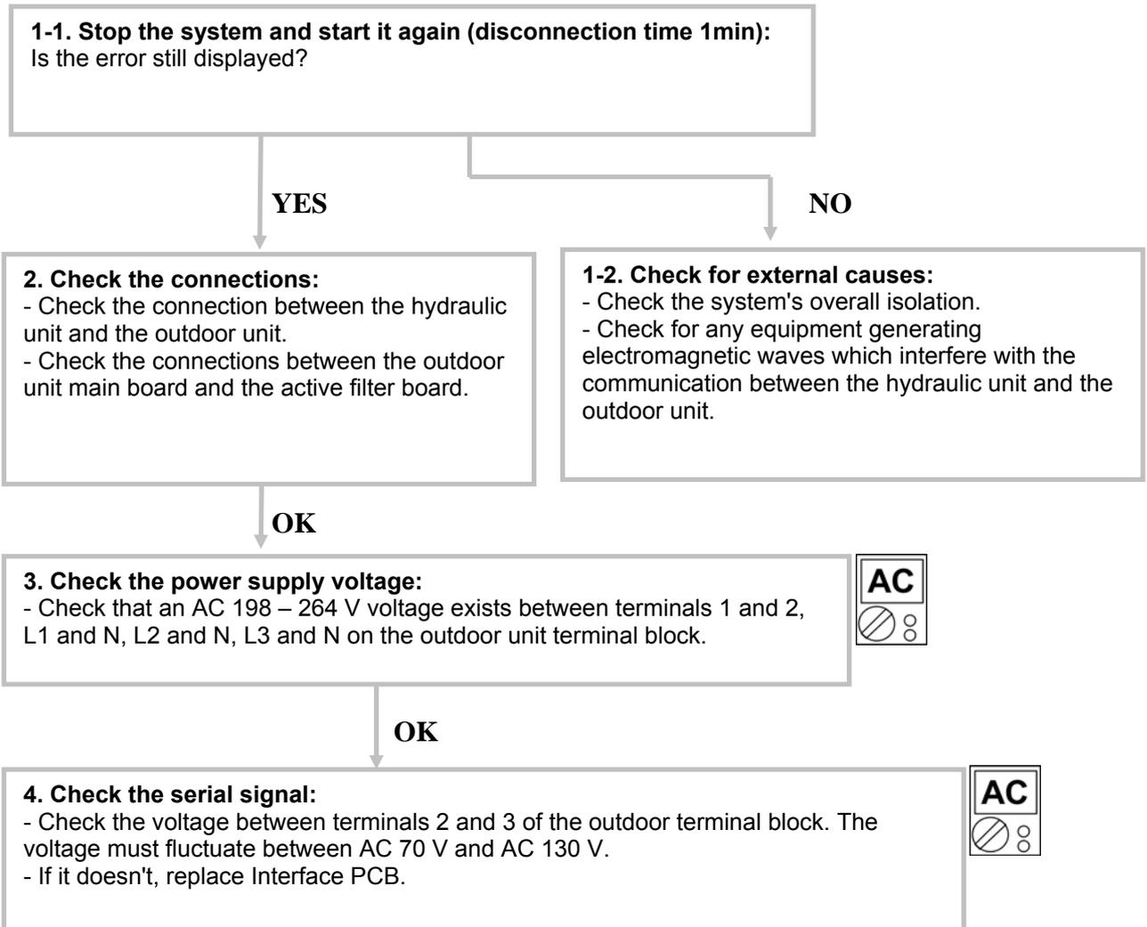
**Clear 4: Heat pump capacity signal error**
