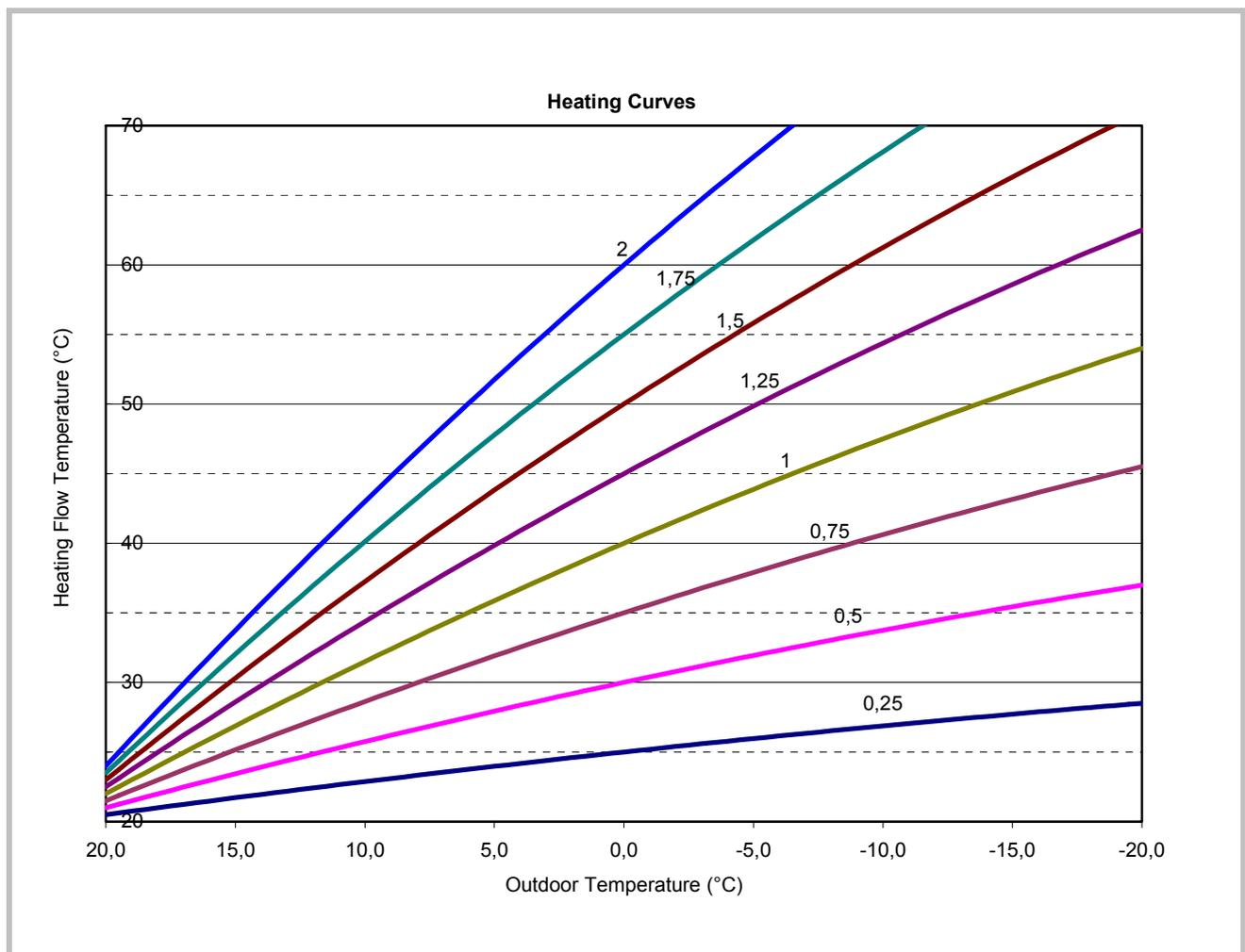
**Heating curve displacement**
