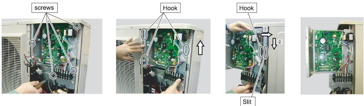
Remove the 4 mounting screws
