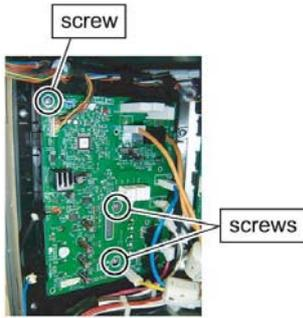
Remove the connectors and screws.
