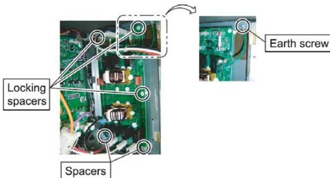
Remove the connectors, locking spacers, spacers, and earth screw.
