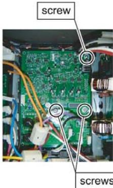
Remove the connectors and screws.
