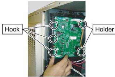
Remove the INVERTER PCB.
