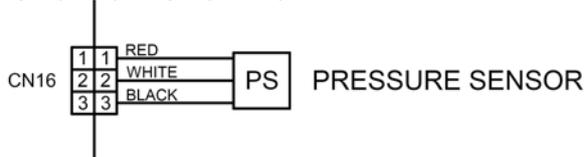
If the voltage is not correct, replace Main PCB.
