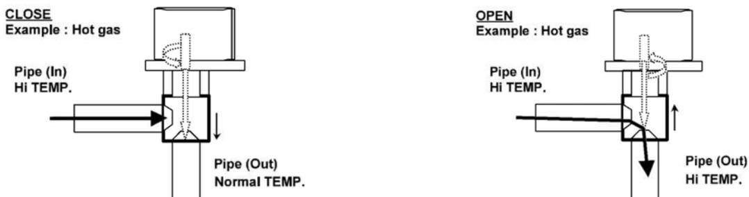
There is no refrigerant flow coming to EEV(INJ) while the liquid injection is inactive. Check whether the liquid injection is active before executing check point 5 for EEV(INJ).
