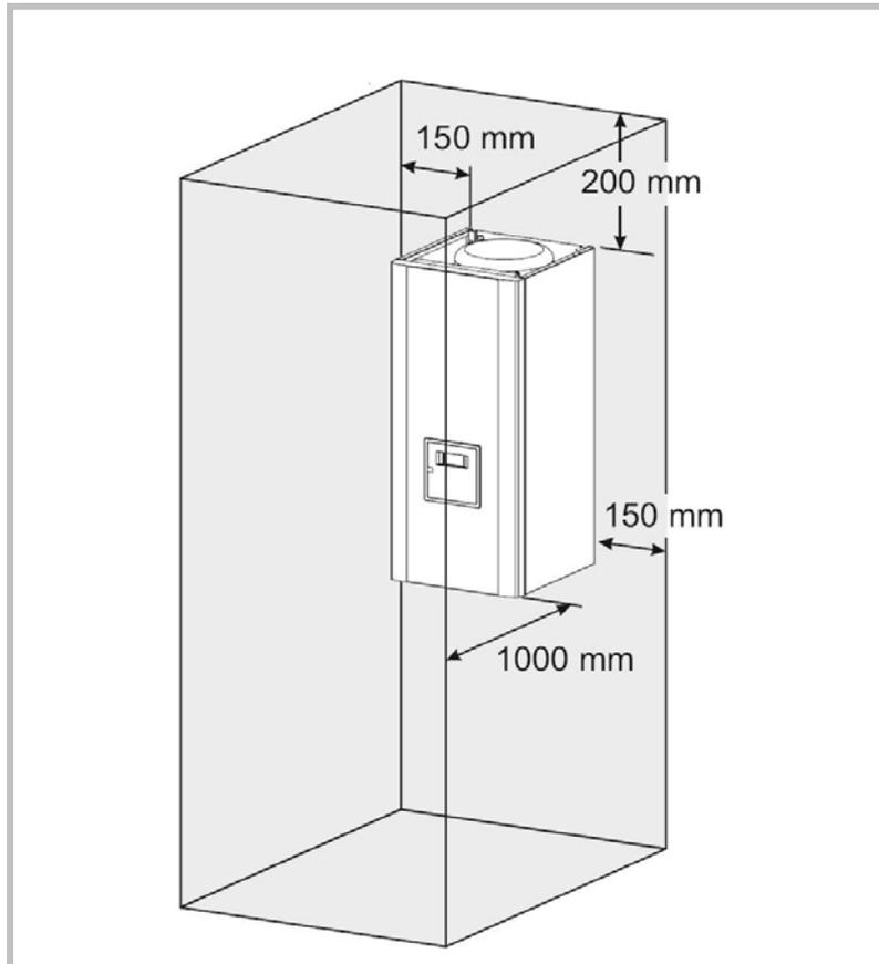
The Hydraulic Unit should be installed in such a way that the distance between the module and the outdoor unit is within the authorized range.
