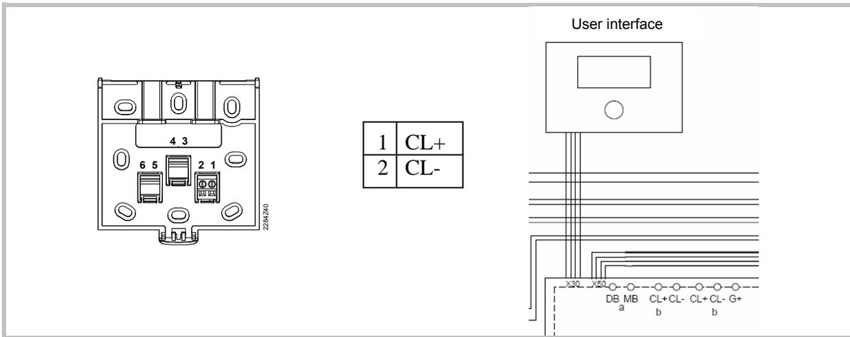
If the installation is equipped with 2 room thermostats, the second thermostat must be connected to the second terminal block b.
