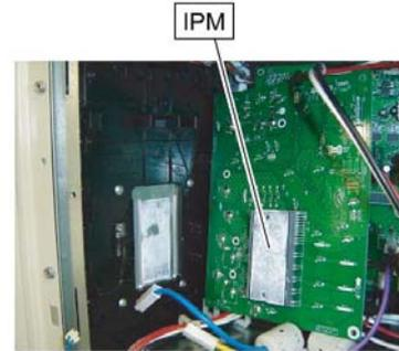
Spread the heat dissipation compound on the other side of IPM when you exchange INVERTER PCB by the repair.
