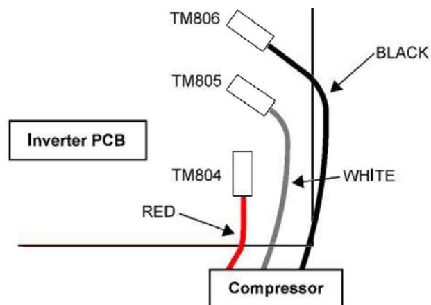
**Check point 2 : check winding resistance**
