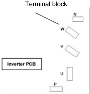
The diagram shows a terminal block with five terminals labeled N, W, V, U, and P. A box labeled 'Inverter PCB' is connected to the W, V, U, and P terminals. A line points from the text 'Terminal block' to the top of the terminal block.
