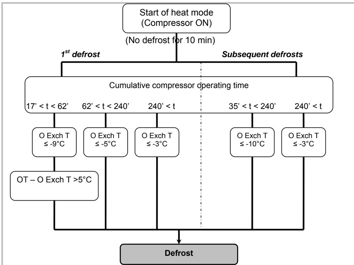
O Exch T : outdoor unit exchanger temperature
